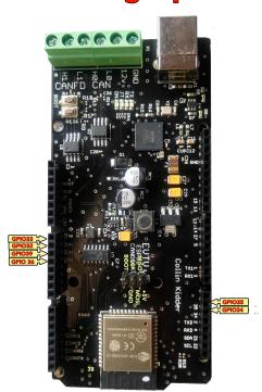
This statement configures the resolution for ALL 7 channels of ADC1 as 12 bit or 4096 resolution. Note that there is also an ADC2 series of channels, but they are almost never used as they are shared with the WiFi function of the ESP32.
