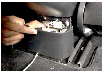
2. Disconnect connector 0x930 by pressing the small white tab and separating the connectors.
