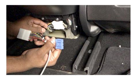
3. Insert the harness assembly connectors into each of the two 0x930 connectors.
